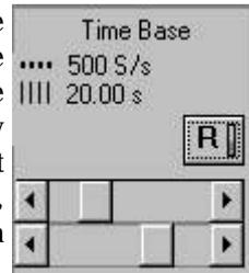
You can turn the Roll Mode on by pressing the button located above the time base control.
