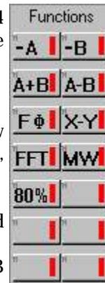
You can turn the function on either by clicking on the channel button or clicking on the function button. Using the first way you turn off the whole channel; however using the other way you turn off just the function and measuring on channel keeps running.
