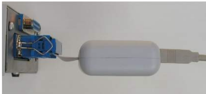
Fig.1.2.5.1: How to connect the USB adapter
