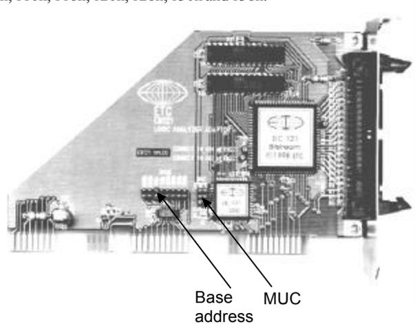
**WARNING: Never install two Base Address jumpers. It can cause a device malfunction.**
