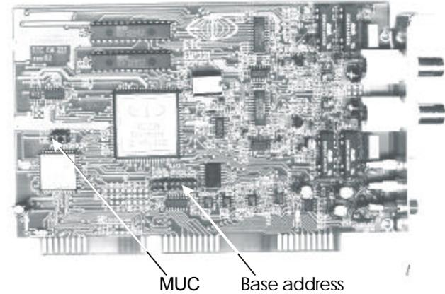
To set the MUC you can install any combination of up to three jumpers on the EM221 add-on card in the MUC part. The jumpers represent the following values (from left to right): 4, 2, 1. To set the specific MUC, please, see the following table:
