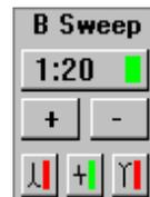
to be displayed on the oscilloscope screen. Default setting is 400 samples from 8000. This is indicated in the upper part of the B Sweep window by 1:20 label, because just 1/20 of stored samples is displayed. By clicking the “+” or “-” buttons it is possible to change the display ratio from 1:2 to 1:20 (See tab. 3.2.10)
